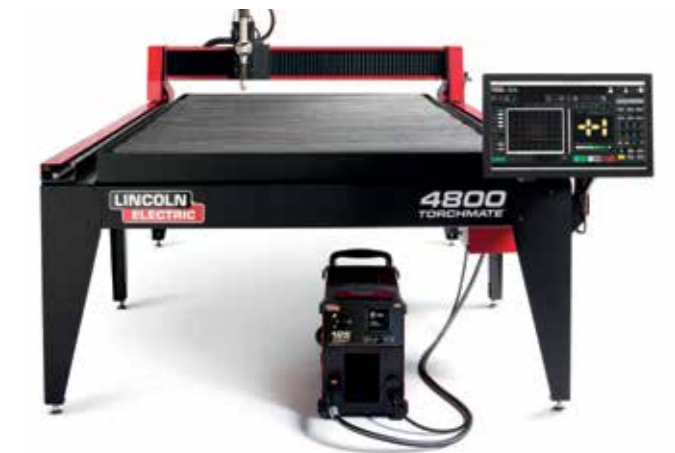
TORCHMATE 4800 | max. cutting range 1.250 x 2.500 mm
